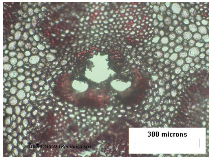
Figure 3 Vascular bundles with two isolate fibre bundles in Bambusa sp.
